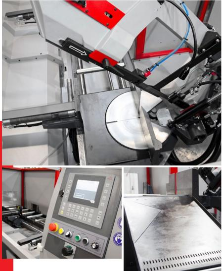
The automatic cutting pressure regulation automatically adapts the cutting feed and pressure to the material. The result is higher cutting output and longer service life.
