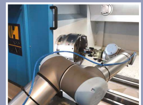
Hydraulic chuck in cooperation with robot
