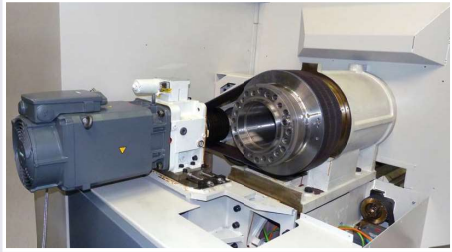
Direct spindle drive with automatic, programmable planetary gearbox.
