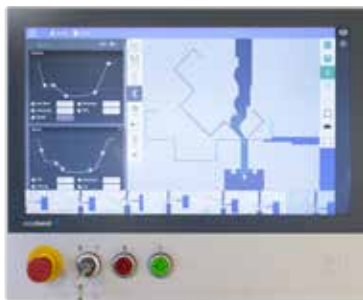
Intuitive Interface with combined numerical-graphical user interface
