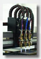
The integrated **PTHC torch lifter** unit controls the cutting height by means of a brushless servo motor During the cutting process, the PTHC unit measures the Arc Voltage and adjust the Z-axis to maintain a constant cutting height, This results in optimum cutting parts.
