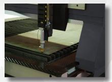
The VULCAN's gantry can be equipped with one ore more Oxy-fule cutting torches.
