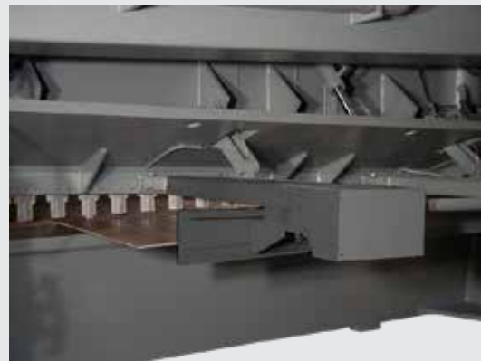
Optional 'heavy duty' hydraulic swing-up (= HDSUB) back gauge stroke 1250 mm.
