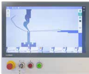
STEP PREVIEWER: bar with possibility of horizontally scrolling of the bending steps
