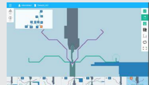
STEP PREVIEWER : bar with possibility of horizontally scrolling of the bending steps
