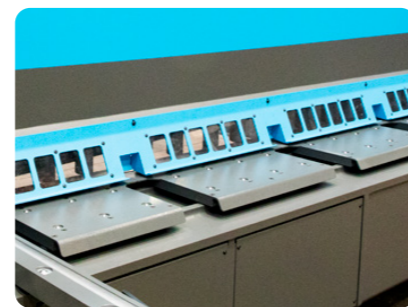
Full table ball transfers mounted in the iron table blocks, for easy feed-in of the sheets.
