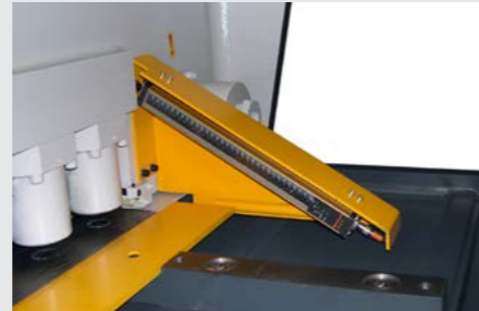
SAFETY LIGHT CURTAIN GUARDS in front of the hold-downs. BALL TRANSFERS mounted in the iron table blocks, for easy feed-in of the sheets.blocks, for easy feed-in of the sheets.
