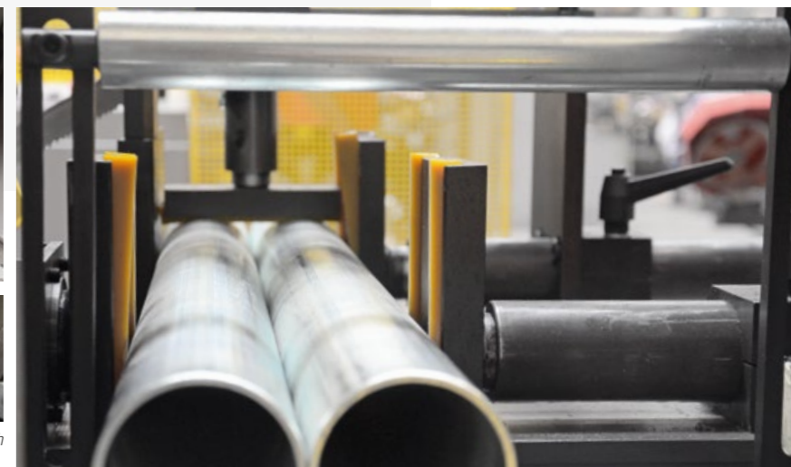
The automatic cutting pressure regulation automatically adapts the cutting feed and pressure to the material. The result is higher cutting output and longer service life.
