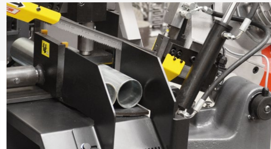
The entire material feeding area is designed as a transit roll-way with embedded rollers.
