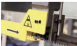
Saw blade guide made of carbide
