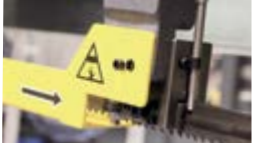
Saw blade guide made of carbide
