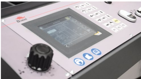
The central panel includes all of the control elements; it is located at an ergonomic height directly at the front of the machine
