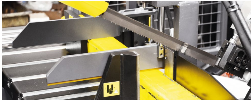
The entire material feeding area is designed as a transit roll-way with embedded rollers
