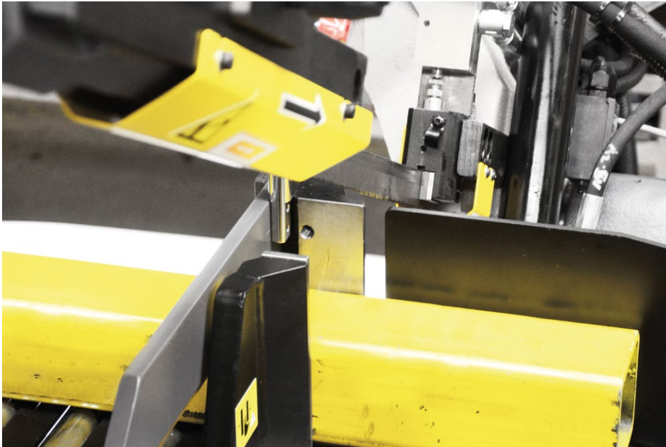
The main vice is designed so that even during angle cuts, which can be adjusted manually up to 45° in the automatic mode, an extremely short 20 mm length of the residual pieces can be achieved
