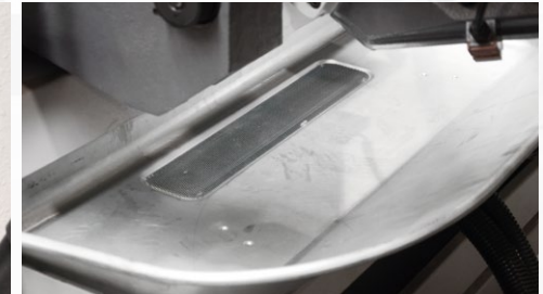
The big, easily accessible chips container provides for their easy removal and prevents unpleasant pools of the cooling agent
