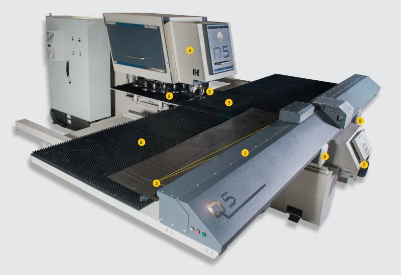
On the large standard brush tables, various workpieces can be nested on standard sheet sizes. The fast AC-servo driven X- and double Y-axis with resp. stroke of 2540 by 1524 mm (100" by 60") or 3000 by 1524 mm (120" by 60") and 3 hydraulic sheet clamps with minimal 'dead zone' 225 by 95 mm (8.85" by 3.74") ensure the highest accuracy on all workpieces (optional CNC moveable)
