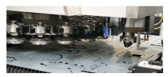
The punch-holder is clamped automatically into the punching head during the tool change. A hydraulic quick-clamping-system is pulling the punch-holder into the punching head, by which the lower part of the punching head (ram) is a mechanical gauge, thus avoiding clearance between punch holder and punching head. While punching, the punch holder and punching head are always connected. The stripper, which is fixed to the punch holder, has two functions:
