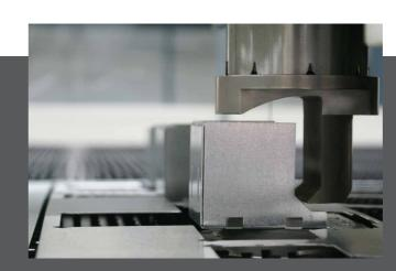
The Q5: exceptionally fast forming capabilities. With a bending height of 75mm (3.0 Inches) in a variety of angles and even on parts which are nested in other locations than 0°-45° and 90° your punch press becomes a multifunctional part processing machine.
