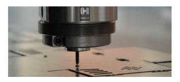
Traditional float tapping or rigid tapping with interpolation, your choice. With the Q series single head punching machines you can use the traditional float tapping system, using a special tap holder. This special float tapping holder will generate the down and up movement for the tap while the C1 axis generating the tap rotation.
