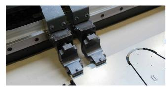
Optionally the clamps are set automatically according to the CNC program, minimizing clamp dead zones. When changing production from full size to small sheets, clamps settings can be made automatically without the risk of operator mistakes and without wasting operator time.
